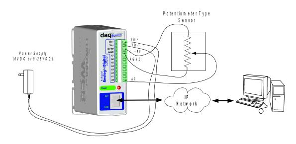
Potentiometer based sensors have three connections: power, ground, and output. Typically, the +5V reference from the Analog Module, and the Agnd are used for power and ground (note that the 5V reference is a very low power output so make sure sensor(s) don't draw more than the rated current output). The output
