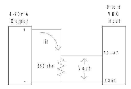
For sensors that have an output of 4-20mA a resistor value of 250 ohms can be used to get the desired output voltage between 0 and 5 volts.
