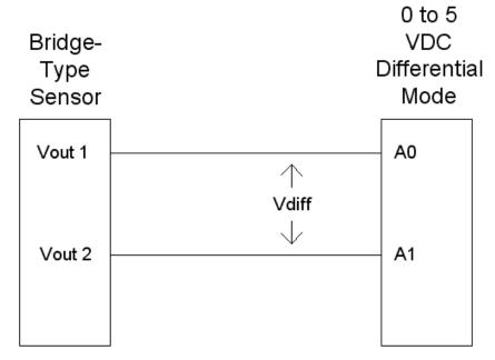
The illustration above consists of a bridge-type sensor with two output signals. The outputs are connected to inputs 0 and 1 of the Analog Module. These two inputs have been placed in differential mode through the
