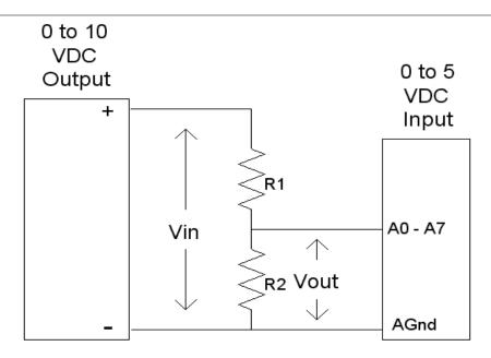
Generally, you can choose a 1K Ohm resistor for R2 and then calculate the value of R1 using the following formula.
