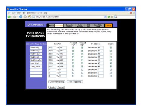
An example screenshot of a gateway router configuration is given below. This setup allows seven ControlByWeb™ products to be accessed on a private network behind a gateway router. Note that this screenshot is simply an example of a typical router setup page. Routers will vary.
