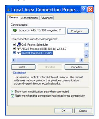
Step 5: Before making any changes to the network settings, write down the current settings so they can be restored once WebRelay-Quad™ is configured. Next, select the radio button labeled "Use the following IP address," and type in the IP address 192.168.1.50. Type in a subnet mask of 255.255.255.0. Leave the default gateway field blank. Click OK to apply settings.
