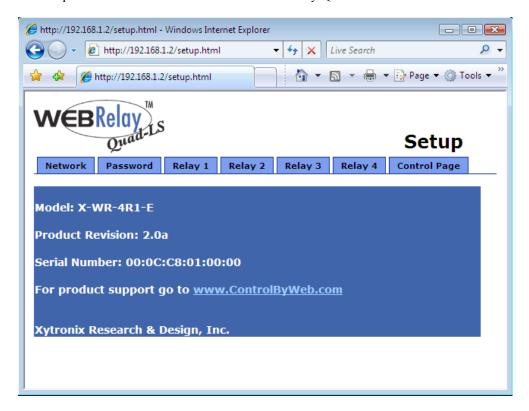
Navigating between setup pages is done by clicking on the tabs at the top of the page. All setup pages require a password. The default password is 'webrelay' (no quotes, all lower case) and no user name is required.
