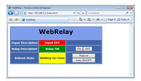
Input Description and Input State: The state of the optically-isolated input can be displayed on the control page. This may be useful to monitor the electrical state of a device. Most reboot applications will not use the optically-isolated input so it can be disabled in the setup so that it is not displayed.
