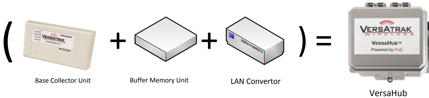
**Includes power supply for all components via Ethernet cable (POE)**
